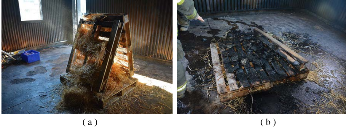
Figure 50. Photographs of wood pallets and straw: (a) before and (b) after the burn (Test 1).
