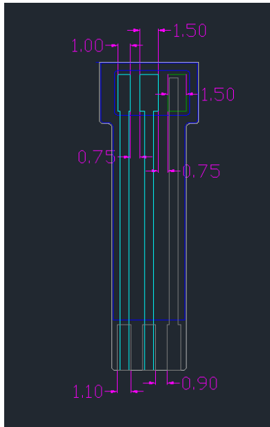
(b) Design 2 –Working Electrode Larger than Counter Electrode.
