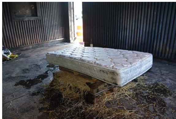
Figure 53. Photographs of a mattress on wood pallets and straw before the burn (Test 2).
