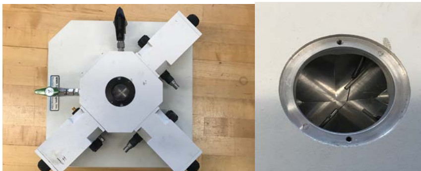
Figure 23. The probe station. The heating stage is inserted from the top left corner of the main body (not shown). In the close up of the observation port, the probes can be seen.
