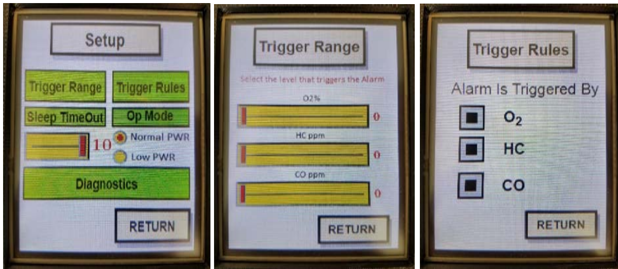
(a) (b) (c) Figure 30. LCD screens: a) Setup, b) Trigger Range, c) Trigger Rules.
