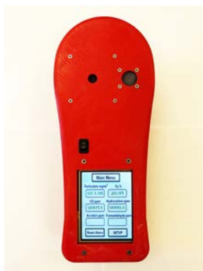
Figure 64. A hand-held particulate and toxic-gas sensor device (Prototype I).
