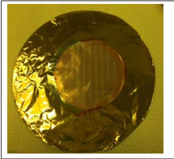
Figure 16. Unmounted PET substrate held down flat using Kapton tape prior to being introduced into sputtering machine.
