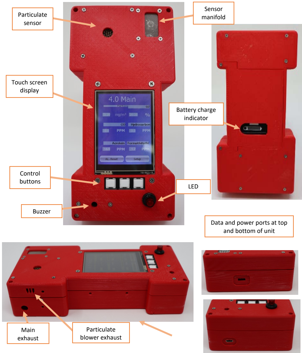
Figure 47. Prototype II as fabricated.
